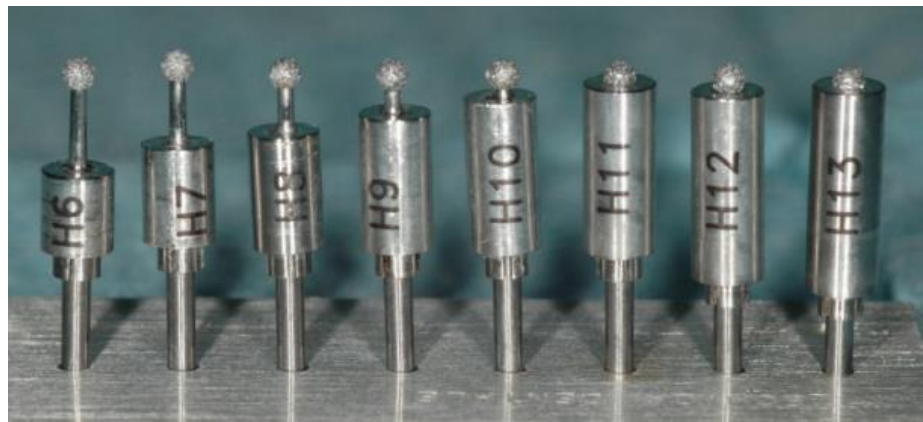
Figure 2: Series of stops linked to the burs by a clip positioned in the crestal part of the drill.
